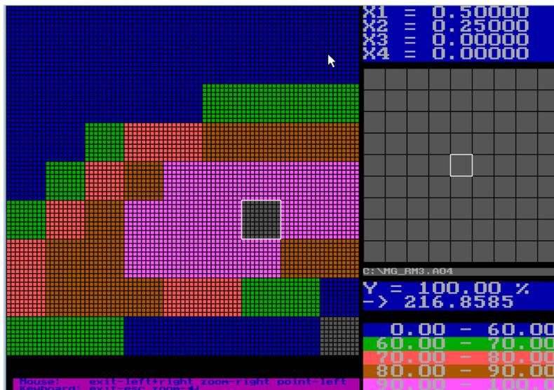
Distribution of tensile strength for the second adequate model depending on the percentage of aluminum and lithium in the alloy.
