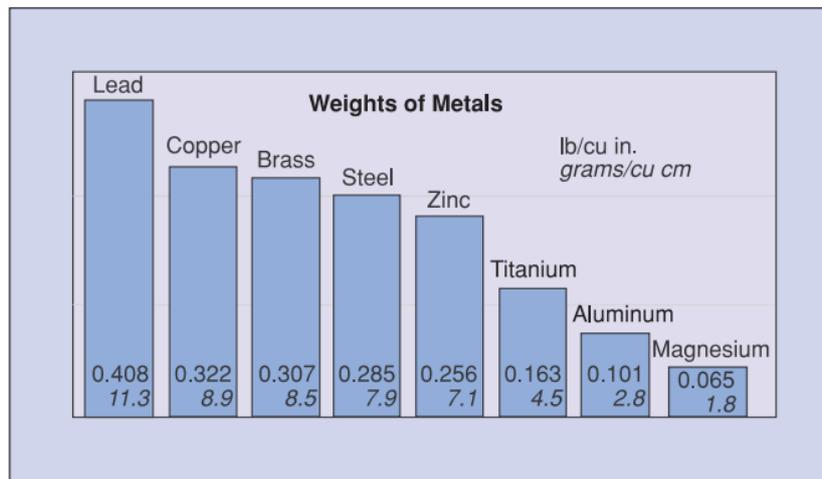
Fig. 1. Magnesium's light weight has allowed it to become the alloy of choice for a number of new markets and applications, such as the automotive, power tool, computer and electronics industries.
